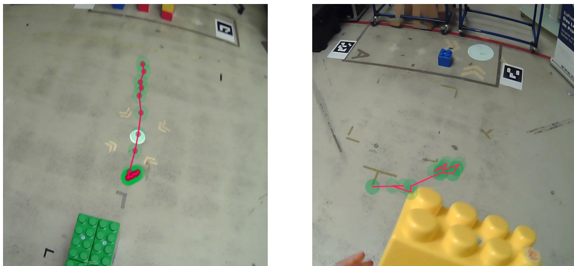
Figure 1: World camera view of eye-tracking device and visualisation of gaze locations per video frame, highlighted in red. The projected moving white circle denotes both the direction and position. The left image represents without, and the right under cognitive load situation.
