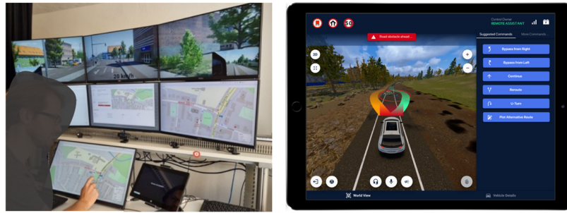
Figure 2: Illustration of different approaches for RA prototypes. Left: multi-monitor workstation with detailed situations and a touch-based interface by Schrank et al. (2024). Right: High-level user interface for a simplified HMI where only the most critical information and suggested maneuvers are displayed by Tener and Lanir (2023).
